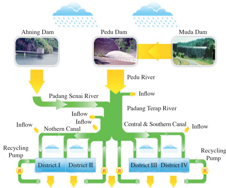
Figure 3. Schematic of irrigation water sources and distribution in MADA
