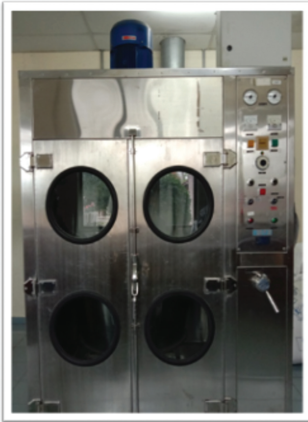
Rajah 6.2: Batch type Fluidized Bed Dryer
